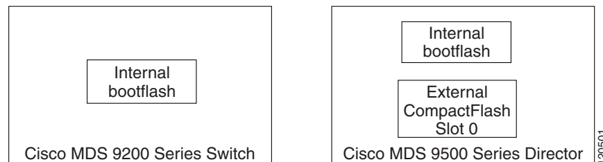
Figure 16-1 Flash Devices in the Cisco MDS 9000 Supervisor Module
