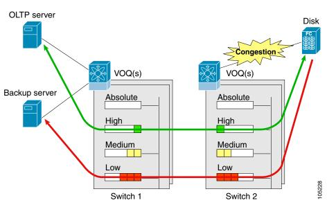
In Figure 2-1, the OLTP traffic arriving at Switch 1 is marked with a high priority level of throughput classification (class map) and marking (policy map). Similarly, the backup traffic is marked with a low priority level. The traffic is sent to the corresponding priority queue within a virtual output queue (VOQ).
