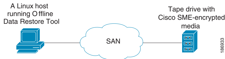
Figure C-1 Offline Data Restore Tool (ODRT) Topology
