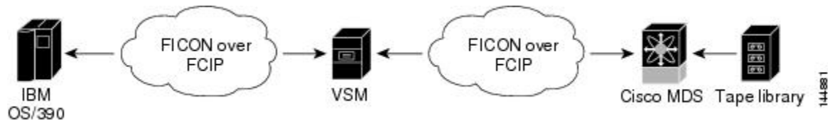
Figure 60: Host Accessing Standalone IBM-VTS (Virtual Tape Server)/STK-VSM (Virtual Shared Memory)
