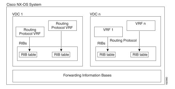
A VRF represents a Layer 3 addressing domain. Each Layer 3 interface (logical or physical) belongs to one VRF. A VRF belongs to one VDC. Each VDC can support multiple VRFs. For more information, see Chapter 12, "Configuring Layer 3 Virtualization."
