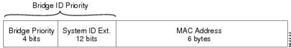
Figure 6: Bridge ID with Extended System ID
