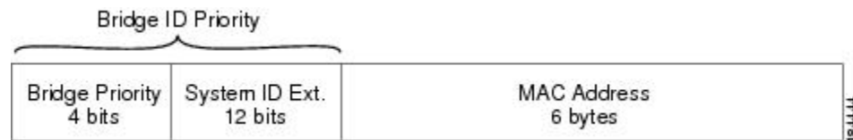
Figure 14: Bridge ID with Extended System ID
