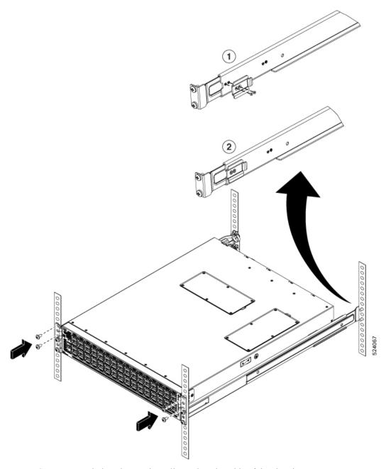
c) Repeat Step 7 to attach the other retainer clip on the other side of the chassis.
