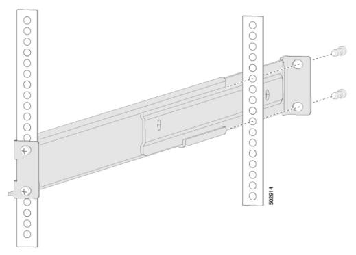
c) Repeat Step 3 to attach the other slider rail to the other side of the rack.
