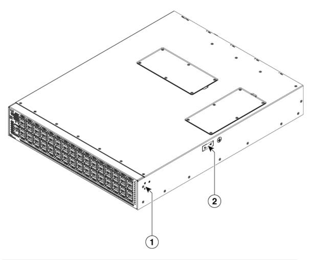
Screw holes for front mounting brackets (both left & right sides)
