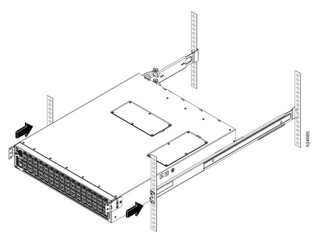
**Step 6** Rotate one front mount bracket to align with the rack (see the following figure).
