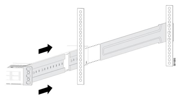
b) Align the two rear rack-mount guides on either side of the switch with the slider rails installed in the rack. Slide the rack-mount guides onto the slider rails, and then gently slide the switch all the way into the rack until the front rack-mount brackets come in contact with two rack or cabinet posts.
