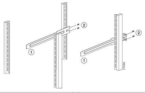
Slider rail with screw holes aligned to screw holes in 2 Two customer-supplied 12-24 or 10-32 screws used to attach each slider rail to the rack
