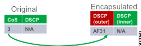
Figure 35: Copy of Priority from Layer-2 Frame to VXLAN Outer Header
