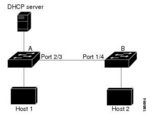
DAI depends on the entries in the DHCP snooping binding database to verify IP-to-MAC address bindings in incoming ARP requests and ARP responses. Make sure to enable DHCP snooping to permit ARP packets that have dynamically-assigned IP addresses.
