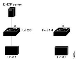
**Step 1** Configure the access list to permit the IP address 10.0.0.1 and the MAC address 0001.0001.0001, and verify the configuration.
