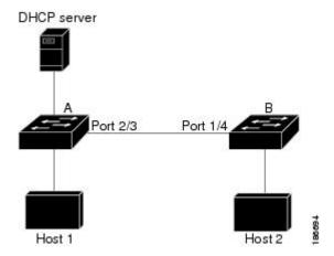
If you configure interfaces as trusted when they should be untrusted, you may open a security hole in a network. If device A is not running DAI, host 1 can easily poison the ARP cache of device B (and host 2, if you configured the link between the devices as trusted). This condition can occur even though device B is running DAI.
