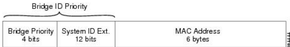
Figure 4: Bridge ID with Extended System ID
