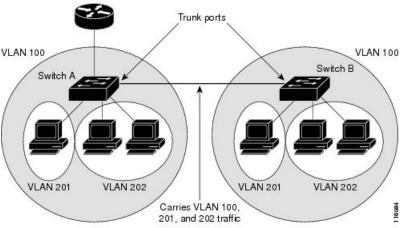
VLAN 100 = Primary VLAN VLAN 201 = Secondary isolated VLAN VLAN 202 = Secondary community VLAN Private VLANs are supported in transparent mode for VTP 1, 2 and 3. Private vlan is also supported on server mode for VTP 3. If we have a server client setup using VTP 3, private vlans configured on the server should be reflected on the client.
