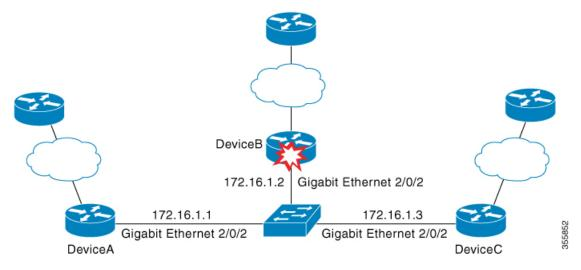
When Gigabit Ethernet 2/0/2 on DeviceB fails, BFD will no longer detect Device B as a BFD neighbor for DeviceA or for DeviceC. In this example, Gigabit Ethernet 2/0/2 has been administratively shut down on DeviceB.
