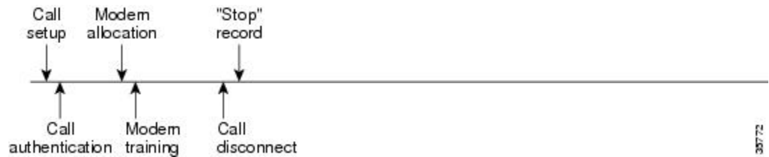
Figure 3: Modem Dial-In Call Setup Sequence With Call Disconnect Occurring Before User Authentication and With Resource Failure Stop Accounting Enabled
