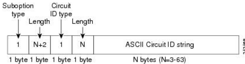
Figure 6: Suboption Packet Formats, Circuit ID Specified
