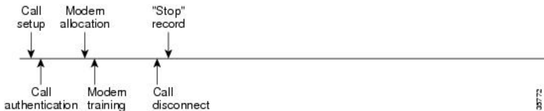
Figure 48: Modem Dial-In Call Setup Sequence With Call Disconnect Occurring Before User Authentication and With Resource Failure Stop Accounting Enabled
