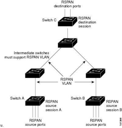
source device must have either ports or VLANs as RSPAN sources. The destination is always a physical port,
