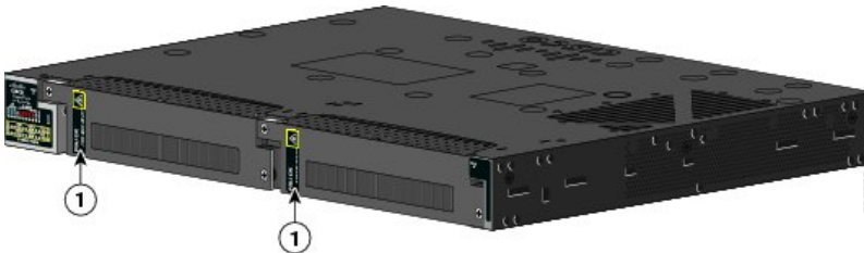
Figure 27: Insert the Power-Supply Module
