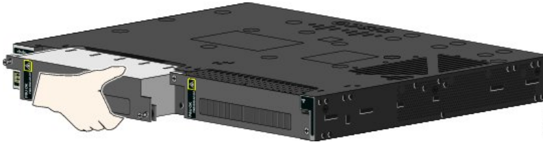
Figure 26: Removing the Power-Supply Blank
