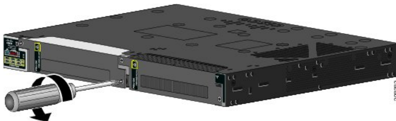
Figure 25: Loosening the Screws on the Power-Supply Blank
