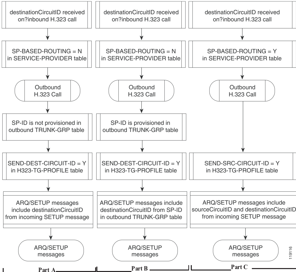
Figure 3-2 H.323 Tandem Calls with Circuit Information Sent
