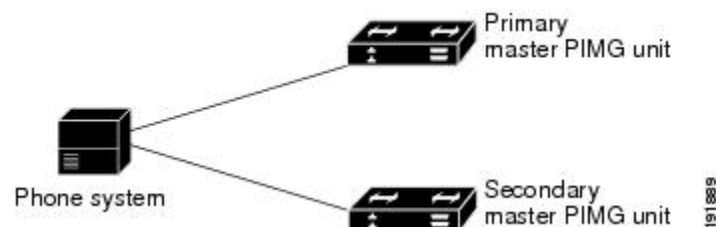
Figure 10: Figure A-7 Serial Cable Connections from Multiple Serial Ports on the Phone System to the Serial Ports on the Master PIMG Units
