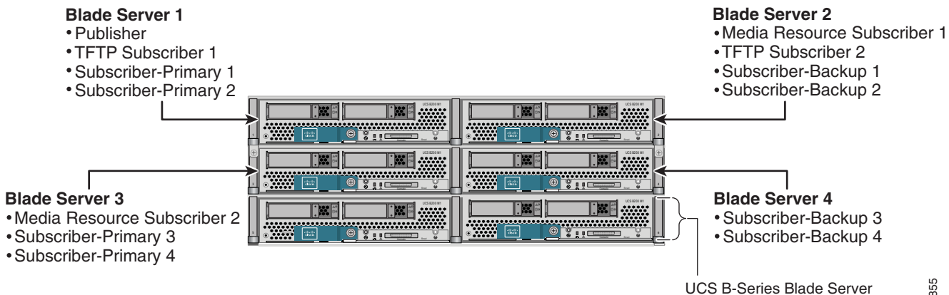
Figure 8-8 Unified CM Server Node Distribution on UCS
