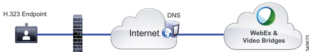
Figure 11-19 Cisco WebEx Meeting Center Video Conferencing Architecture Using H.323 Video Without a Call Control System
