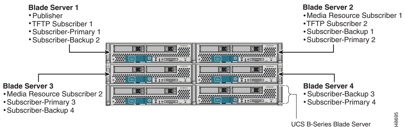
Figure 9-8 Unified CM Server Node Distribution on UCS
