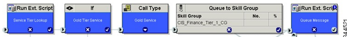
Figure 2: Changing a Call Type Prior to the Queue to Skill Group Node
