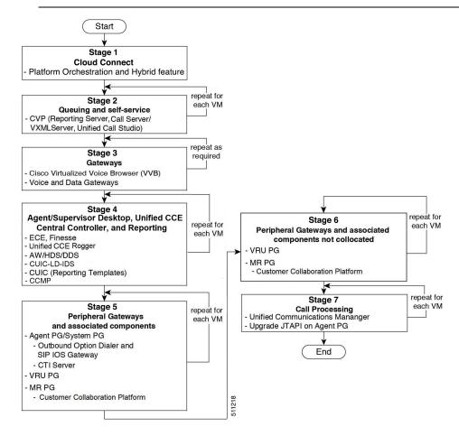
The following diagrams illustrate the stages of the component-level upgrade flows for the Packaged CCE 2000 Agent Deployment solution upgrade. Each diagram covers one of the stages. The letter at the end of each flow indicates the start of the next flow that you are required to perform.
