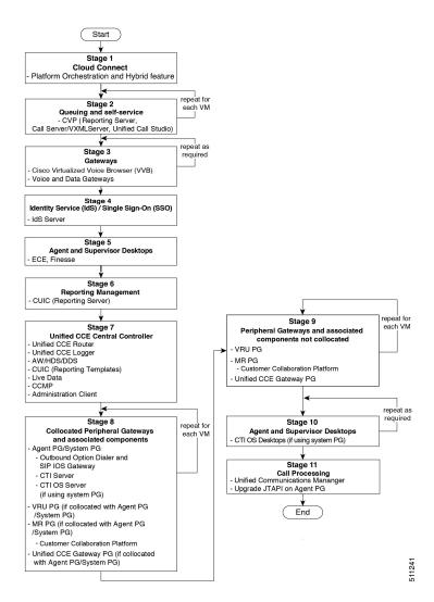
The following diagrams illustrate the stages of the component-level upgrade flows for the Packaged CCE 4000 Agents and above Deployment solution upgrade. Each diagram covers one of the stages. The letter at the end of each flow indicates the start of the next flow that you are required to perform.
