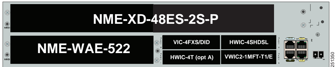
Figure 4 Interface Card and Service Module Configuration On a Cisco 3925
