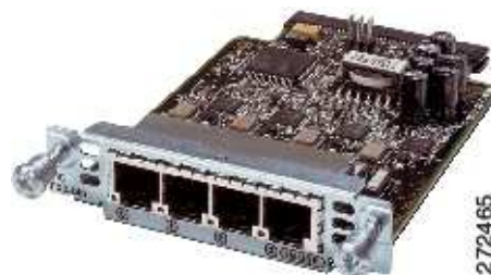
Figure 56 Four Port FXS/DID Voice Interface Card
