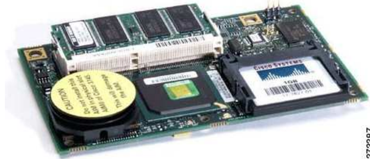
Figure 55 Cisco Unity Express Advanced Integration Module
