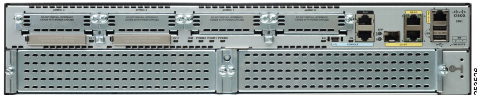
Figure 3 Interface Card and Service Module Configuration on a Cisco 2951 Router
