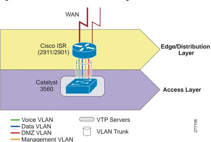
Figure 23 shows VLAN trunks that are defined for the Streamlined Small Branch LAN.
