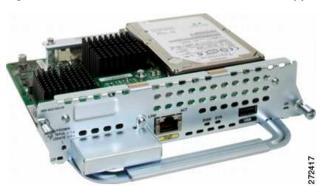
Figure 57 Cisco NME-WAE-502 Wide-Area Application Engine
