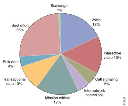
Figure 29 Bandwidth Allocation for Eight-Class QoS Model
