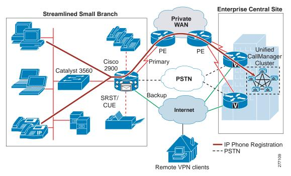
Under normal operations shown on the left in Figure 46, the branch office connects to the central site via a WAN, which carries data traffic, voice traffic, and call signaling. IP Phones at the branch exchange call signaling information with the Cisco Unified CM cluster at the central site. The voice gateway in the router forwards both types of traffic (call signaling and voice) transparently and has no "knowledge" of the IP Phones in the branch.
