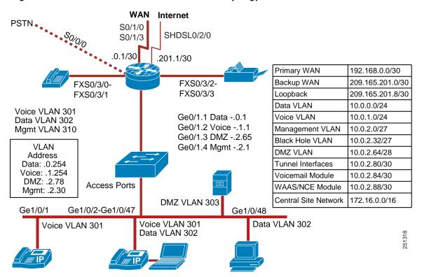
Figure 2 Streamlined Small Branch Network Topology
