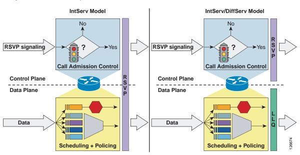
Figure 53 RSVP Operational Models: IntServ and IntServ/DiffServ
