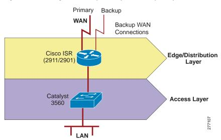
Figure 25 High Availability and Rapid Recovery Components
