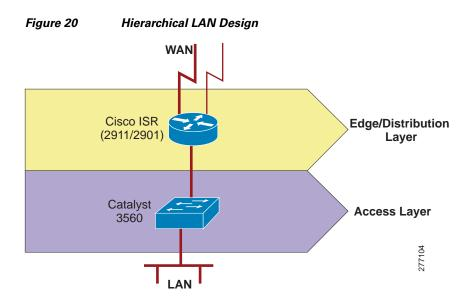
Switches must support many features to facilitate interoffice connectivity. Features of the Catalyst 3560 switch that were leveraged by the Streamlined Small Branch Network are described in the following sections:
