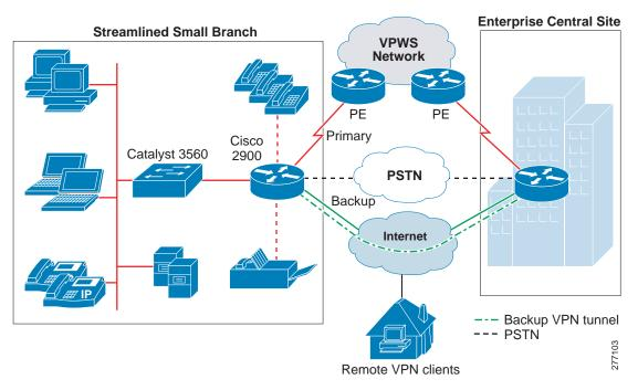
VPWS services allow the enterprise to keep its existing WAN infrastructure and to transparently connect to the service provider's Ethernet network, providing a transparent migration path to VPLS services. The leased-line connections to the PE device continue to use the typical Layer 2 encapsulation mechanism:
