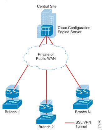
Figure 42 Deployment of CCE in the Streamlined Small Branch Network.
