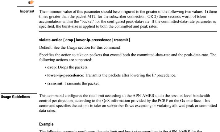
The following example configures the rate limit and burst size according to the APN-AMBR for the uplink direction. Policing is done for the traffic based on PCRF value recieved and traffic is dropped as the violate action is specified as drop.
