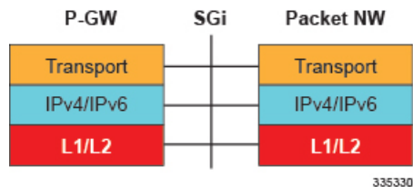
Figure 30: Protocols Supported on the SGi Interface
