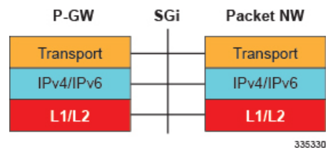
Figure 30: Protocols Supported on the SGi Interface
