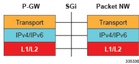
Figure 19: Protocols Supported on the SGi Interface
