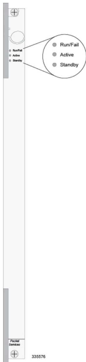
Figure 53: Packet Processing Card LEDs
