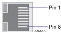
Figure 31: SPIO Ethernet RJ-45 Interface
