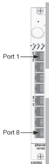
Figure 41: Fast Ethernet Line Card Interface Connectors
