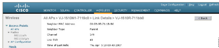
Figure 8-29 All APs &gt; Access Point Name &gt; Link Details &gt; Neighbor Name Page
