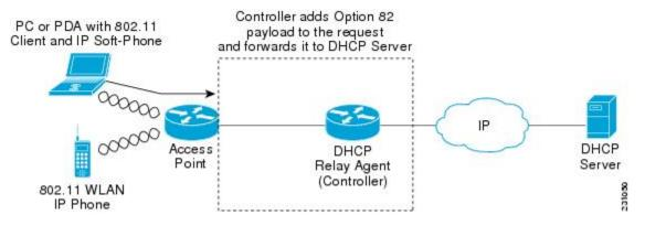
The access point forwards all DHCP requests from a client to the controller. The controller adds the DHCP option 82 payload and forwards the request to the DHCP server. The payload can contain the MAC address or the MAC address and SSID of the access point, depending on how you configure this option.
