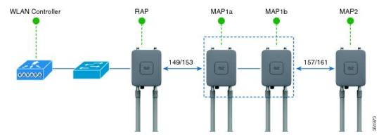
High gain directional antenna must be used in typical serial-backhaul deployments. Additionally, preferred parent configurations must be used to create serial-backhaul mesh networks.
