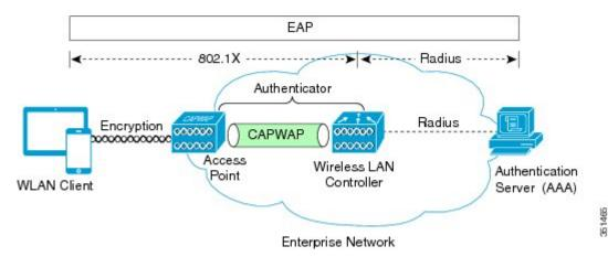
802.1X is an IEEE standard for port-based network access control and was adopted by the 802.11i security standard workgroup. The 802.1X standard provides authenticated access to 802.11 wireless LAN networks using the following logic:
