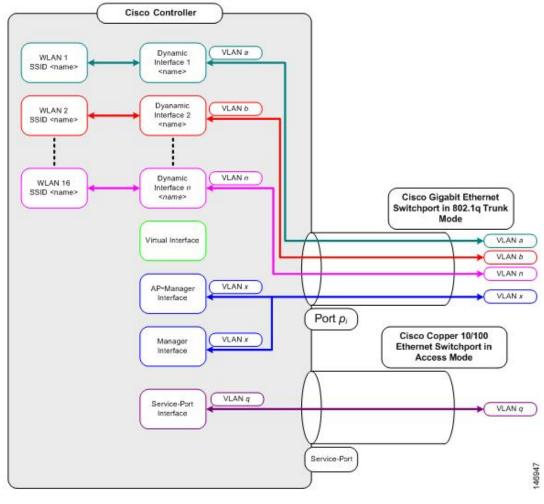
Figure 17: Relationship between Ports, Interfaces, and WLANs
