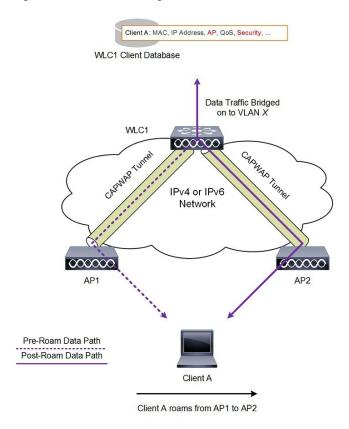
When the wireless client moves its association from one access point to another, the controller simply updates the client database with the newly associated access point. If necessary, new security context and associations are established as well.
