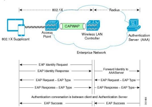
EAP as defined by RFC 3748 supports four packet types as part of the EAP authentication process:
