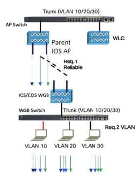
The Receiver address (RA) of legacy broadcast packet is FF:FF:FF:FF:FF:FF and there will not be any retransmission if the packet is lost in the air. The reliable downstream broadcast feature replaces this RA with WGB address and Destination address (DA) with special multicast address 01:00:5e:80:xx:xx. This will make the packet as a unicast packet and enables ACK mechanism. The packet will be retransmitted when the ACK is not received.
