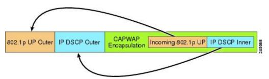
For CAPWAP control traffic the IP DSCP value is set to 46, and the 802.1p user priority is set to 7. Prior to transmission of a wireless frame over the backhaul, regardless of node pairing (RAP/MAP) or direction, the DSCP value in the outer header is used to determine a backhaul priority. The following sections describe the mapping between the four backhaul queues the mesh access point uses and the DSCP values shown in Backhaul Path QoS.
