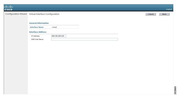
Step 32 In the IP Address field, enter the IP address of the controller's virtual interface. You should enter a fictitious, unassigned IP address.
