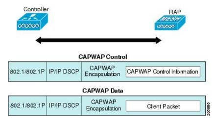
For the backhaul, there is only one type of encapsulation, encapsulating mesh traffic. However, two types of traffic are encapsulated: bridging traffic and CAPWAP control and data traffic. Both types of traffic are encapsulated in a proprietary mesh header.
