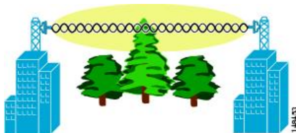
Figure 12: Typical Obstructions in a Fresnel Zone
