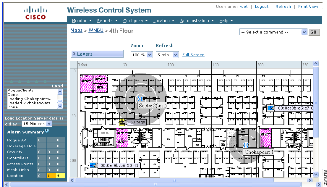
Figure 7-15 New Chokepoint Displayed on Floor Map
