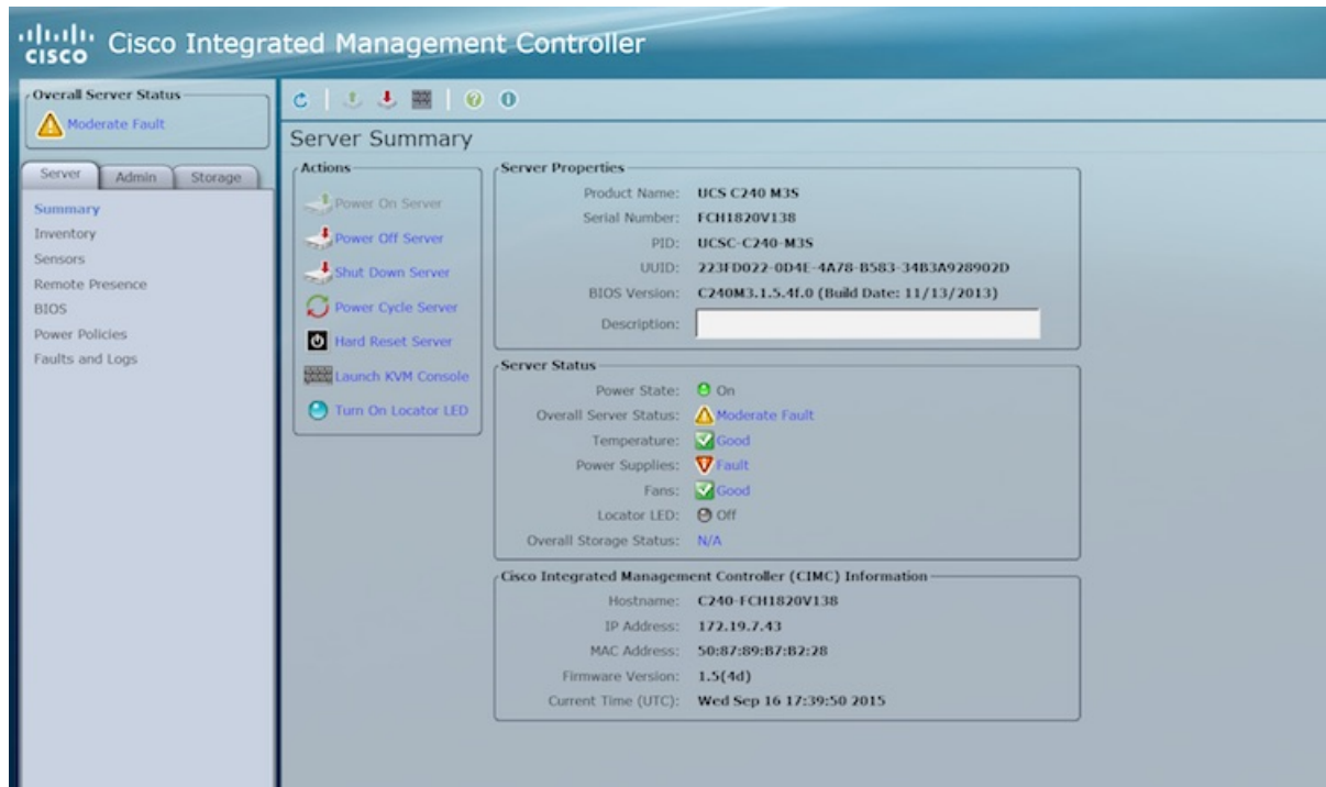
Figure 19: Cisco Integrated Management Controller Interface
