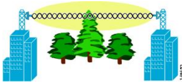
Figure 20: Typical Obstructions in a Fresnel Zone
