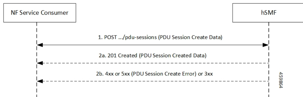
Figure 109: Create Service Operation on hSMF Call Flow
