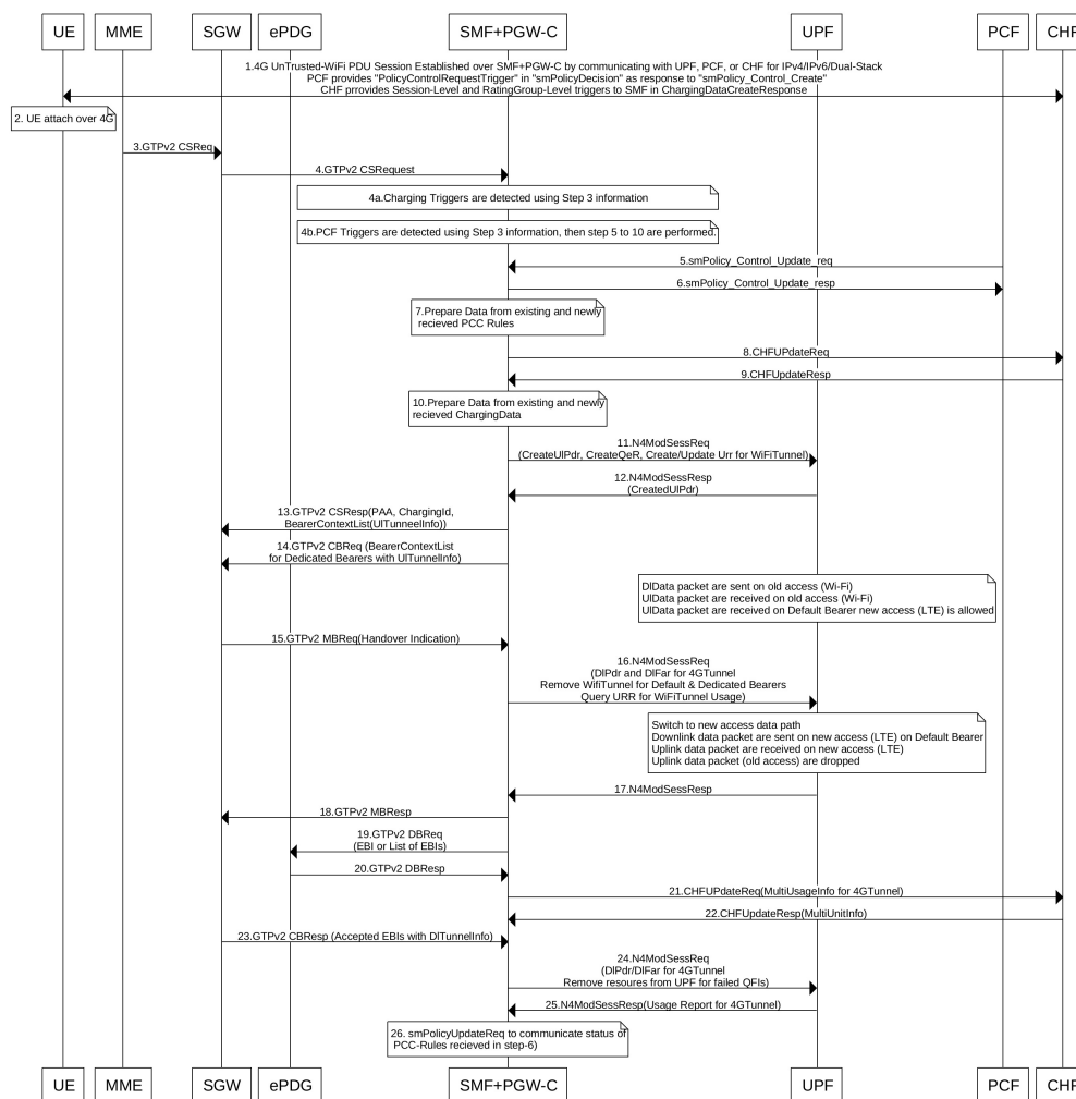
Figure 87: Non-3GPP Untrusted Wi-Fi to EPC Handover Call Flow
