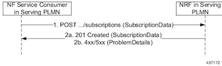
Figure 163: Subscription (POST) Call Flow
