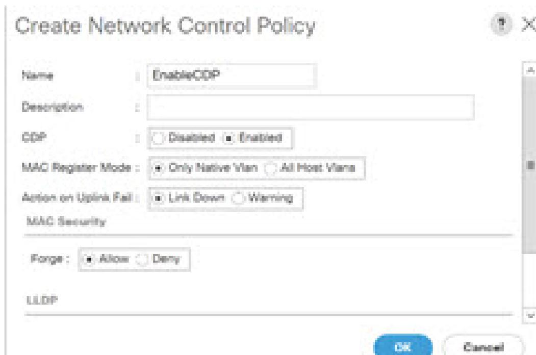
The screenshot shows a 'Create Network Control Policy' dialog box. The 'Name' field is filled with 'EnableCDP'. The 'CDP' section has 'Enabled' selected. The 'MAC Register Mode' has 'Only Native Vlan' selected. The 'Action on Uplink Fail' has 'Link Down' selected. The 'MAC Security' section has 'Forge' set to 'Allow'. There are 'OK' and 'Cancel' buttons at the bottom right.
