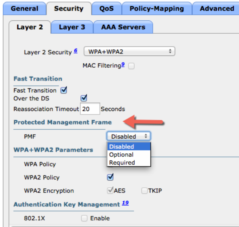
図 11-18 [Security] - [Layer 2] - [Protected Management Frame 1]
