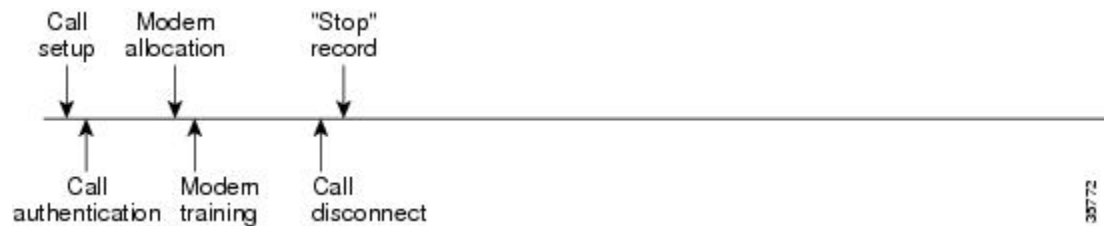
Figure 4 Modem Dial-In Call Setup Sequence With Call Disconnect Occurring Before User Authentication and With Resource Failure Stop Accounting Enabled
