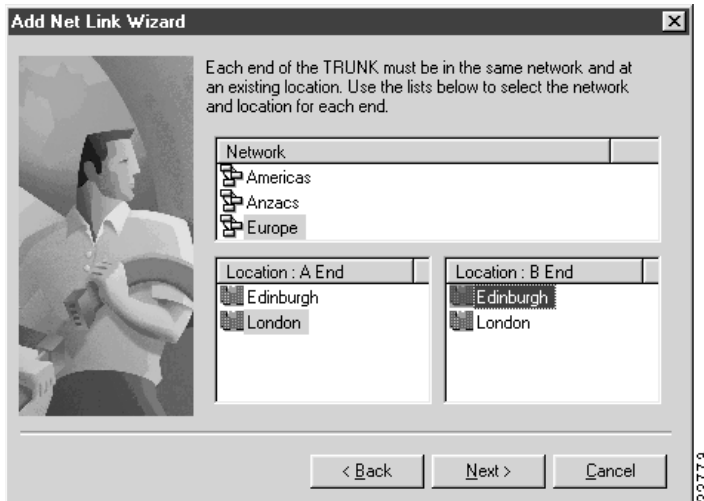
Figure 5-19 Selecting Trunk End Point Locations
