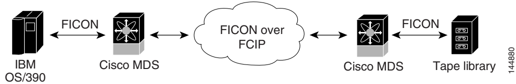
Figure 36-20 Host Directly Accessing IBM/STK (StorageTek) Library
