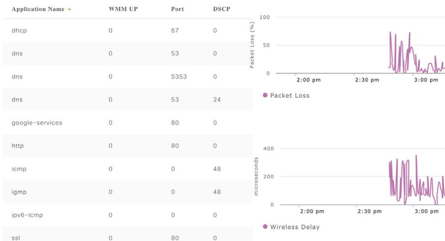
Intelligent Capture helps Nancy conclude that the problem is on the wireless side (as indicated by the high rate of packet loss) and she therefore focuses on troubleshooting the AP to which the user was connected.
