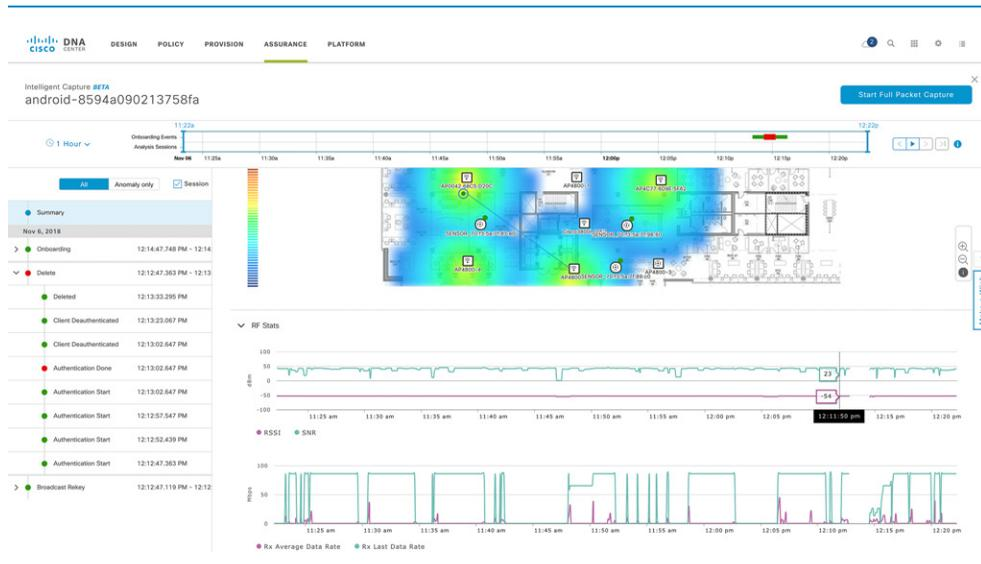
Next Larry zooms into the onboarding failure events and reviews information from the Auto Packet Analyzer that shows details for each onboarding event. This includes handshake information between the AP and the client. This allows Larry to identify the delay, timeout, and re-transmission for each onboarding step. The up and down arrows indicate the direction of the packets between AP and client.
